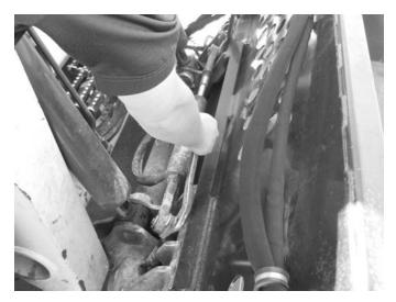
4. Tilt the loader coupler backward a small amount until it is fully engaged in the attachment mounting bracket.
